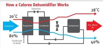
Principles of operation - air to air dehumidifier
