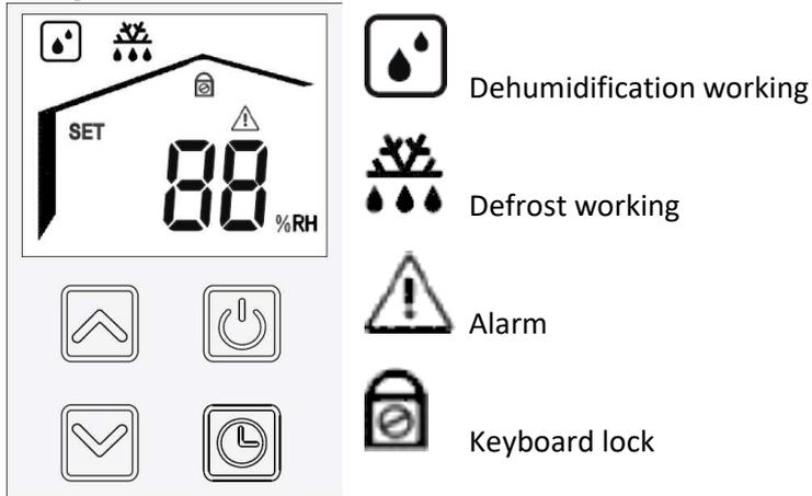
As the humidity sensor of the units needs 15s for heat reflection, when the units start up, users should wait 15s till the units show exact ambient relative humidity.
