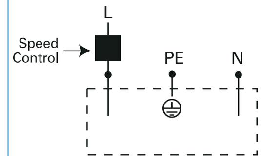
Speed controllers for single phase ebm-papst motors should be installed in the active line in series with the motor.
