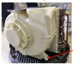
Use a screwdriver to remove the two screws
