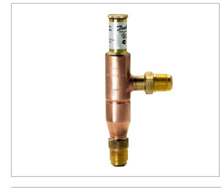
KVC is a hot gas bypass regulator applied for the adaption of the compressor capacity to the actual evaporator load. Placed in a bypass between high and low
