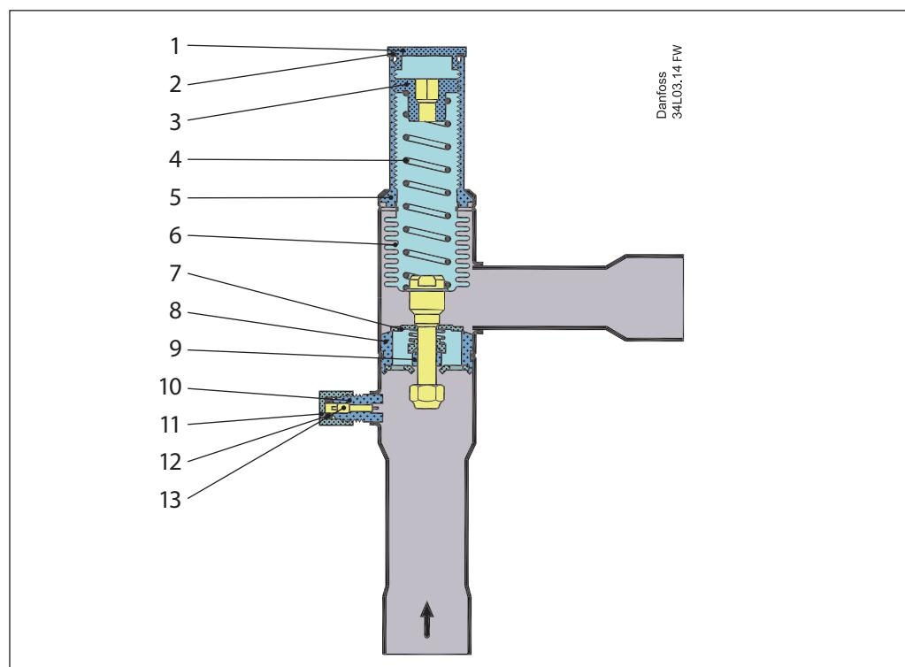
Evaporator pressure regulator type KVP opens on a rise in pressure on the inlet side, i.e. when the pressure in the evaporator exceeds the set value.
