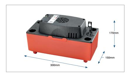
The DiversiTech RedBox 2 Litre Tank Pump is a condensate tank pump with a flow rate of 280 LPH and a lift of 5.1 metres. This pump has metal mounting tabs which allows the tank to be screwed to the wall. The universal power lead makes the pump easy to install, service and retrofit.
