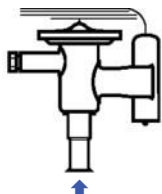
Angle flow (fixed orifice)
