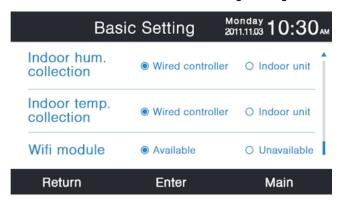
In basic setting interface, press Up/Down key to adjust unit number; press Left/Right key to move the cursor. Some functions are reserved for some models and the information is gray.
